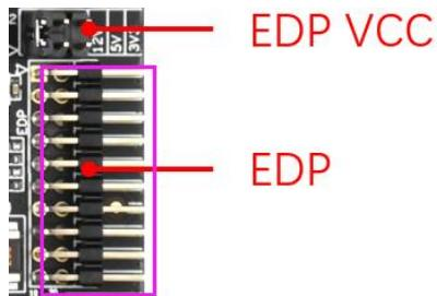
This interface is a common EDP screen interface, in the form of 10 \* 2 double row pins, 3.3V screen power supply. In order to avoid burning boards and screens, please note the following:
