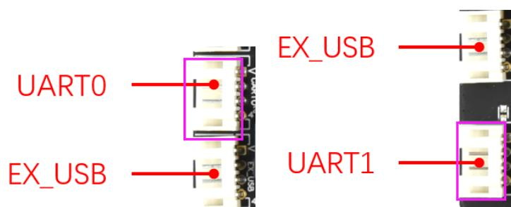
The board have to two sets of ordinary UART serial ports, which can support the UART serial port devices on the market.
