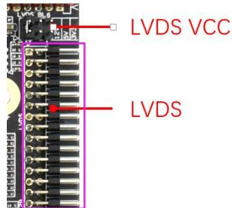
General LVDS interface definition, support single / dual, 6/8 / 10-bit 1080P LVDS screen. The screen voltage can be selected through a jumper cap, and it can be selected to support 3.3V / 5V / 12V screen power supply.
