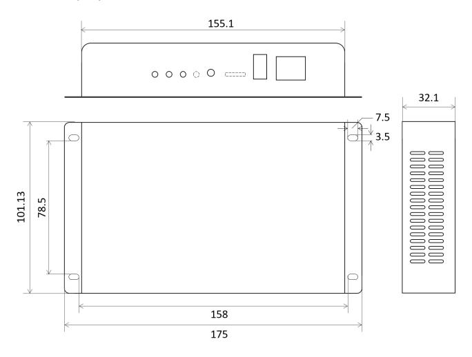
Tolerance: ±0.3 Unit: mm
